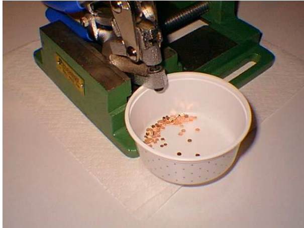
Vise and punch setup for punching pads.
